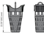
Note: Openings in trash bucket are 74.4"2 (48,028mm2)
